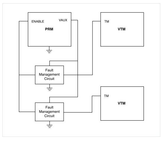
There are many possible implementations of the Fault-Management Circuit. One implementation is shown in Figure 3. This circuit is low cost, uses little board space and satisfies the performance requirements of a broad range of systems. It gets its power and ground from the PRM's VAUX and SGND pin, respectively. The components are off-the-shelf resistors, capacitors and N-channel MOSFETs.
