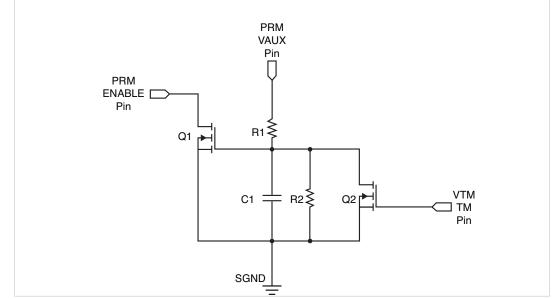
During normal operation, this circuit has no effect: TM is high, keeping Q2 turned on and Q1 turned off. On system start up, the circuit still has no effect. The PRM<sup>™</sup> starts before the VTM<sup>™</sup>, but the RC time constant is long enough to keep the voltage on C1 too low to turn on Q2 before Q1 turns on; otherwise Q1 would turn on, bring ENABLE low and shut down the PRM again.
