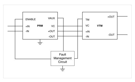
In the case of a series stack of two VTMs, two Fault-Management Circuits would be required, one for each VTM. A block diagram of this circuit is shown in Figure 2. (For the sake of simplicity, only the Fault-Management Circuit connections are shown. These connections would be the same for a series or parallel VTM configuration.)
