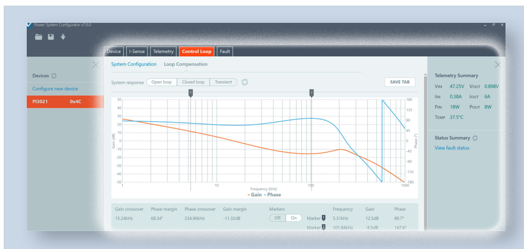
Figure 26 Loop Compensation section of Control Loop tab
